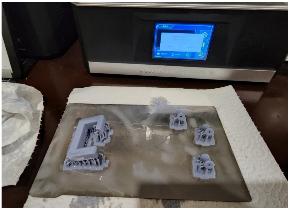
Figure 8: Resin printing of roller frame and roller
